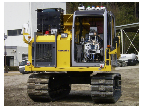
Tele-operated robot for crawler dumps (KuroQ)
