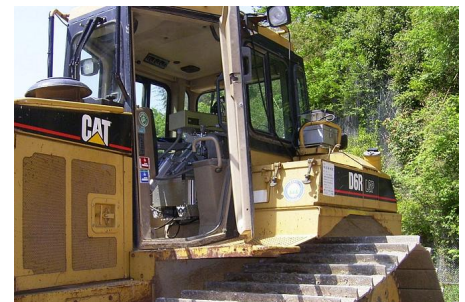
Tele-operated robot for bulldozers (BuruQ)
